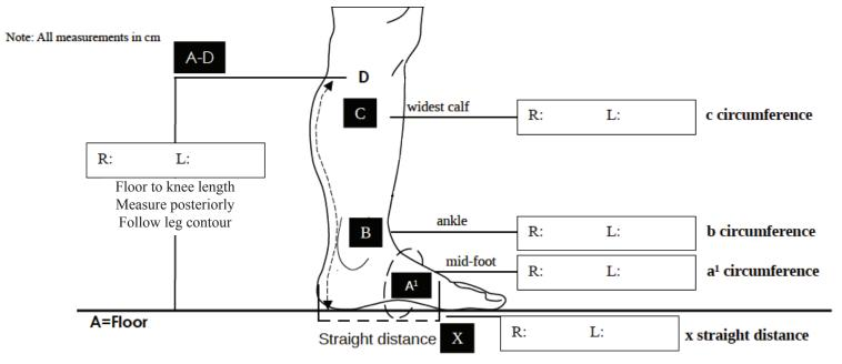
All FarrowWrap Off-The-Shelf legpieces are sized by taking three simple measurements: widest calf circumference (C), ankle circumference (B), and floor to knee crease length (A-D).
